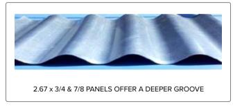
The 2.67"  $\times$  1/2" panel is the most common corrugated metal used today. The 2.67" Denotes the distance from the center of one ridge to the center of the next. The overall height is 1/2". The 2.67"  $\times$  3/4" and 2.67"  $\times$  7/8" panels offer a deeper groove for a more pronounced corrugated style.
